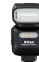
The SB-500 is a compact, lightweight flash. With a guide number of 24/78.7 (m/ft, ISO 100, 23°C/73.4°F), its flash head tilts up to 90° and rotates horizontally 180° for bounce flash which adds natural light. The built-in LED light (with a choice of three output levels) has a color temperature close to sunlight, and can serve as an auxiliary light for both still and movie shooting.
